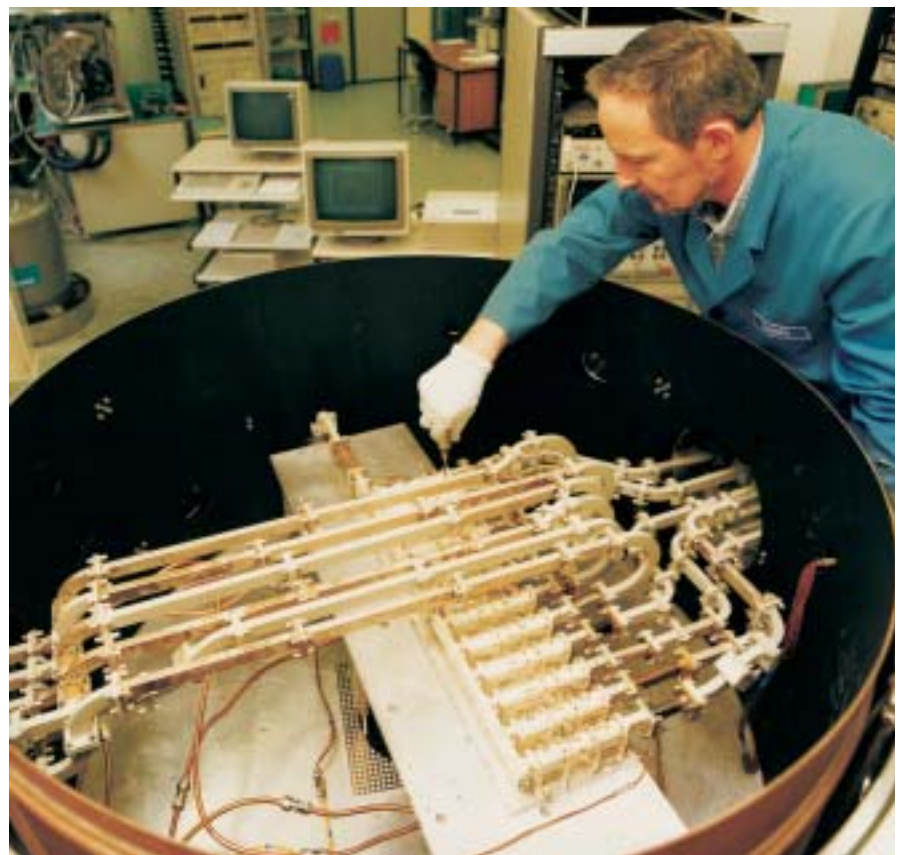
Output multiplexer in thermo vacuum chamber
